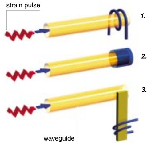
**(Fig. 4)** Comparison of strain pulse converter systems
